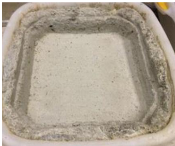
Figure 14. Concrete slab for salt scaling evaluation
